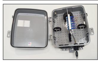
Compact polycarbonate terminal for up to 12 fiber connections with ample slack storage. The OptiTip cable assembly (97-CBLTIP12-LU) is factory terminated as shown.
