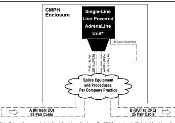
\*Note: Only one line-powered, single-line, AdrenaLine unit is shown. The CMPH supports up to 25 single AdrenaLine units. Express-powered, single-line, AdrenaLine units are equipped with a third wire pair in the cable tail for powering purposes.
