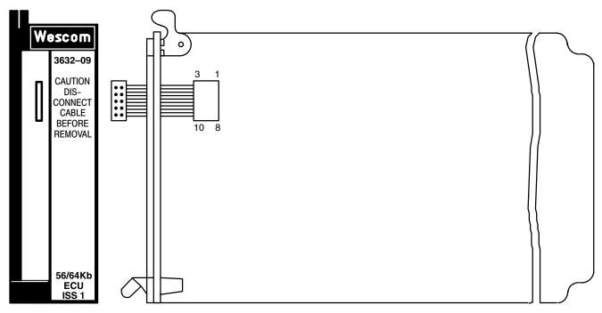
Figure 1. 3632-09 ECU Front and Side Panels
