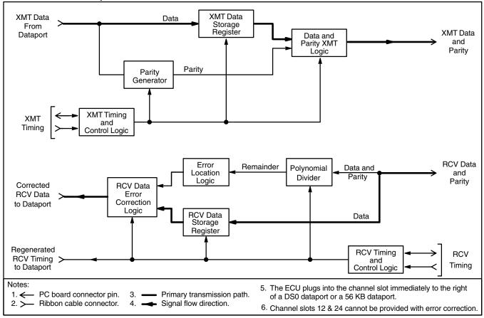
Figure 2. 3632-09 ECU Block Diagram
