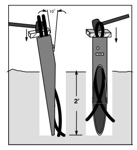
Figure 7. Integral Stake Mounting
