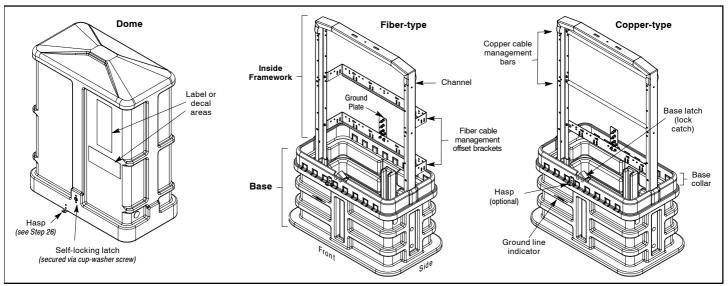
Figure 2. Typical CMPH Enclosures, Dome Removed Views
