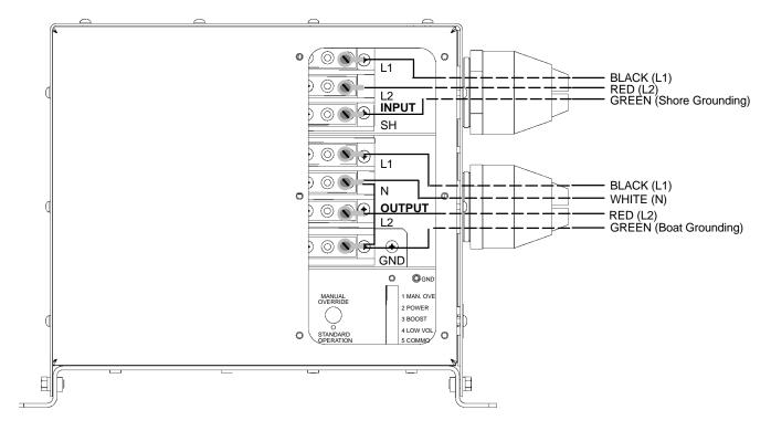
Figure 5. Typical Wiring as an Isolation Transformer – Method 1 (see Figure 1 for Electrical Diagram)
