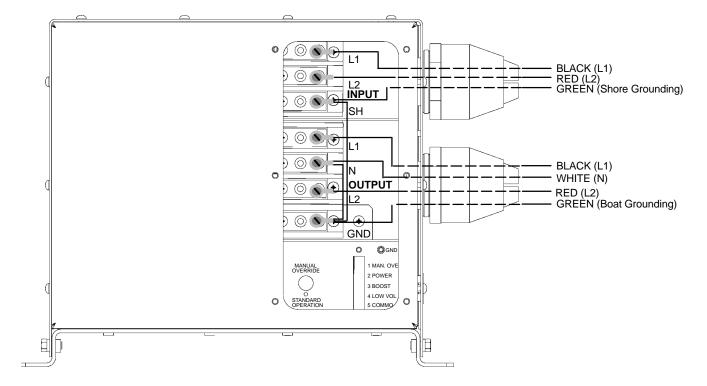
Figure 7. Typical Wiring as a Polarization Transformer – Method 3 (see Figure 3 for Electrical Diagram)
