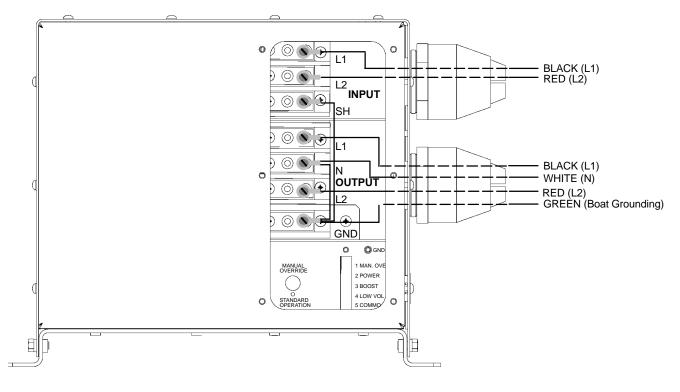
Figure 6. Typical Wiring as an Isolation Transformer with Primary Ground Fault Protector – Method 2 (see Figure 2 for Electrical Diagram)
