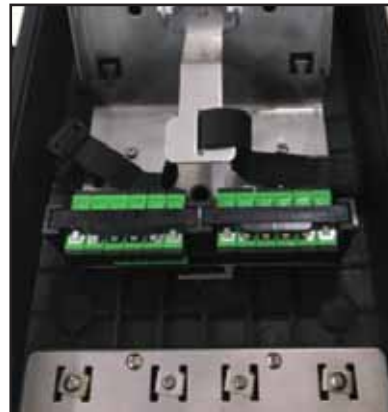
Internal SC Adapter Frame with 16 SC/APC Adapters
